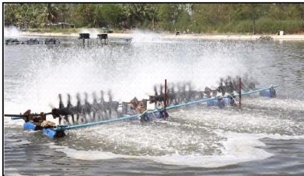
20 to 30 per cent. If initial stocking density is very high, say 100/ $m^2$  it may become essential to provide each such ponds of water spread area of say, 500  $m^2$  with at least two aerators. In such cases, requirement of water exchange too becomes very high. Ponds, where feeding rates are above 40 to 50 kg/ha/d, frequent aeration is needed.
